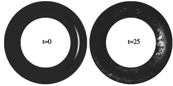
FIG. 1. Impurity distribution projected onto a poloidal cross section (radial dimension not to scale). White: high impurity density. Dark: low impurity density. Left: initial distribution, localized on the outboard midplane (at s=0 ). Right: after 25 time units corresponding to about 100 \mu\text{s} . Parallel transport is slow compared to radial transport. The inward pinch effect is clearly visible.
